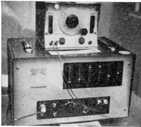
Transistor a.f. generator and transistor frequency meter (0 to 1 Mc/s) shown by S.E.C.R.E.
