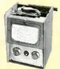
Vacuum Tube Voltmeter TYPE TF 104 F. 25 mV to 300 V (20 c/s to 1,500 Mc/s); 10 mV to 1,000 V d.c.; R from 0.02 \Omega to 500 M \Omega . Optional voltage multipliers.
